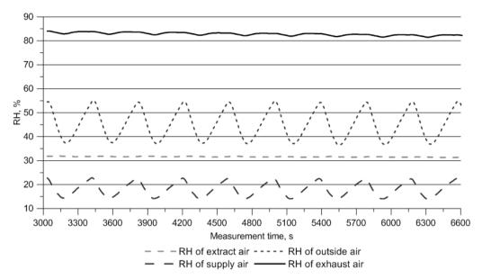
Fig. 3. Sequence of changes in relative humidity of the outside air for the outside air temperature of 5°C and 24°C – temperature of removed air
