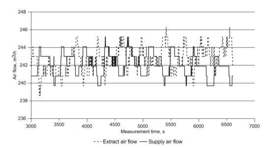
Fig. 4. Sequence of changes of air flow for exhaust and outside air for the outside air temperature of  $5^{\circ}$ C and  $24^{\circ}$ C – temperature of removed air
