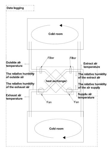
Fig. 1. The scheme of the testing-bench for heat exchangers and construction of the plate heat exchanger
